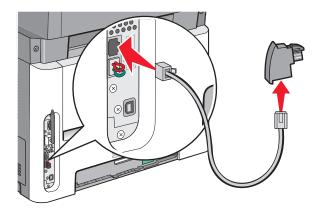
**3** Connect the adapter into the N slot of an active analog telephone wall jack.
