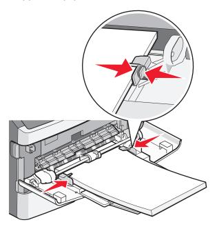
5 Slide the paper gently into the multipurpose feeder until it comes to a stop. Make sure the paper fits loosely and is not bent or wrinkled.
