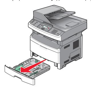
**2** Squeeze and slide the guides to the correct position for the paper size you are loading.
