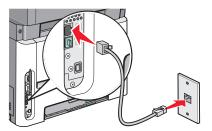
**3** Remove the plug from the printer EXT port  $\widehat{\blacksquare}$ .
