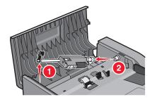
**4** Use a clean, lint-free cloth dampened with water to wipe the separator rollers.
