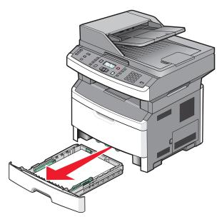
**2** Locate the lever shown, and then pull it down to release and remove the jammed sheets.
