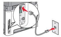
**3** Remove the protective plug from the printer EXT port  $\widehat{\blacksquare}$ .
