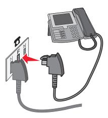
**5** If you would like to use the same line for recording messages on your answering machine, then connect a second telephone cable (not provided) between the answering machine and the other N slot of the active analog telephone wall jack.
