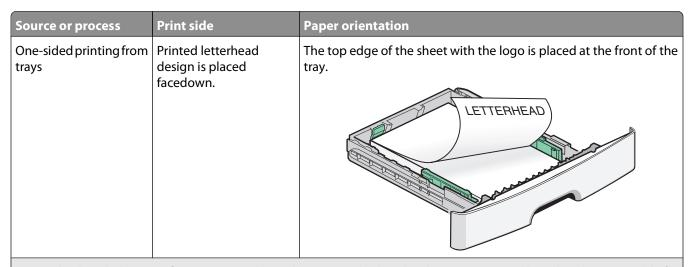
**Note:** Check with the manufacturer or vendor to determine whether the chosen preprinted letterhead is acceptable for laser printers.
