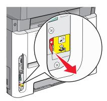
**8** Temporarily connect a USB cable between the computer on the wireless network and the printer.
