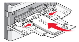
**Warning—Potential Damage:** Never use envelopes with stamps, clasps, snaps, windows, coated linings, or self-stick adhesives. These envelopes may severely damage the printer.
