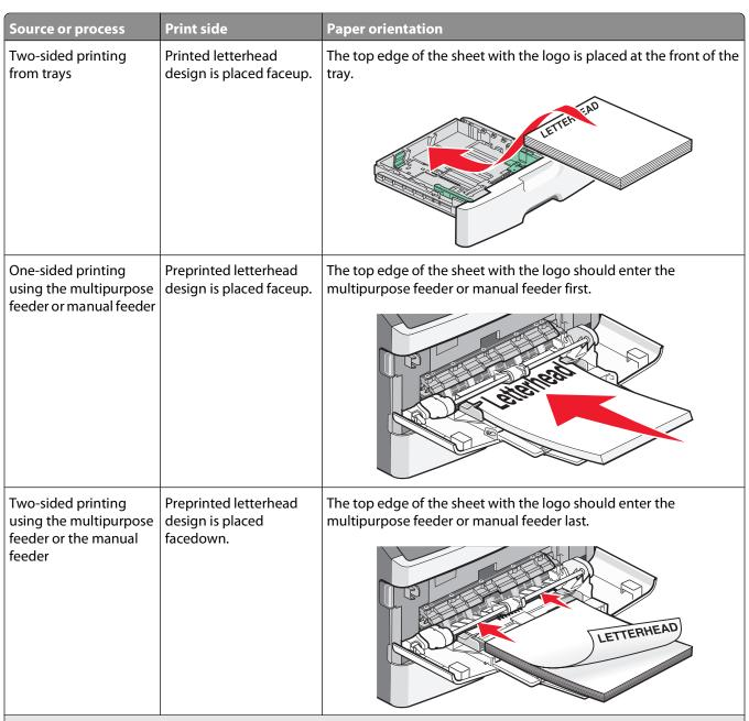
**Note:** Check with the manufacturer or vendor to determine whether the chosen preprinted letterhead is acceptable for laser printers.
