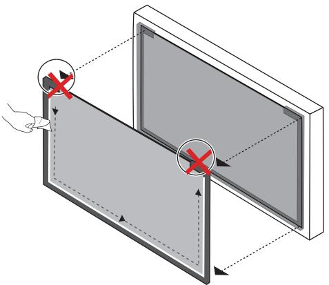
• There is ±3 mm accuracy over 95% of the touch screen. Avoid using the screen out of that area. Note:
